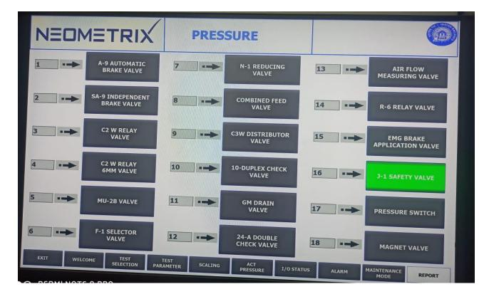
To start a test click on a particular valve as per test setup ready for testing. Now Test can be started by clicking on START button, Test will automatically run for define time and report will be save in PDF format.
