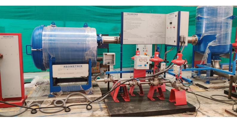
Aircrafts have varying atmospheric pressure conditions as altitude differs. We can create different altitude conditions inside a closed chamber by means of a vacuum pump and set of modulating and flow control valves. This Test Rig was designed for the ground testing of Aerospace Units. The test unit (UUT) will be placed between two chambers one of which is simulating cabin and other is simulating altitude chamber.
