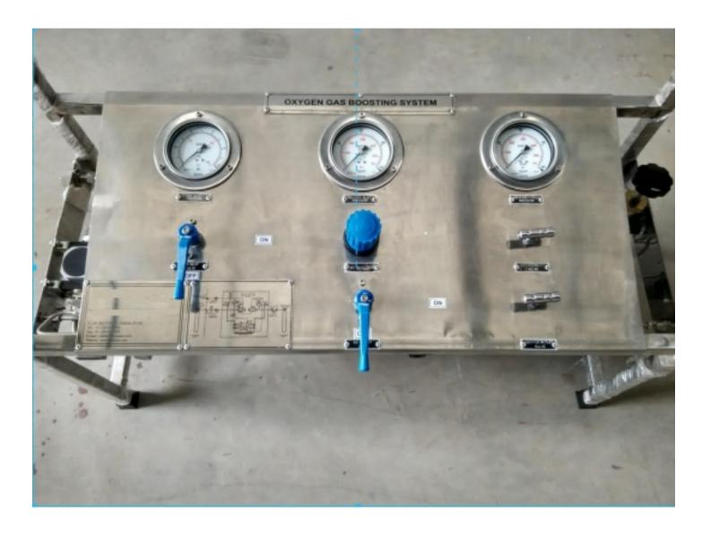
This machine is used to safely boost the oxygen gas up to 350 bar. Our oxygen booster systems and oxygen bottle filling stations provide an efficient, safe and economical way of handling oxygen. In addition to filling oxygen cylinders, these systems can be used in the aviation and aerospace industries for in-flight life support oxygen as well as for gas boosting, gas mixing, SCUBA, Rebreathers and other SCUBA applications in the commercial, military or recreational dive industries
