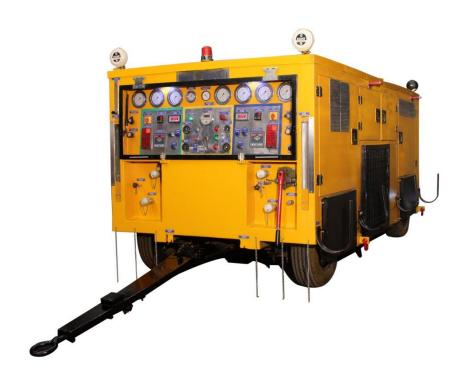
**HST 300U is UNIVERSAL HYDRAULIC SERVICING TROLLEY**. HST 300U is used as Servicing Trolley of the various aircraft. It consists of the following **MAJOR SUBSYSTEMS** as follows:
