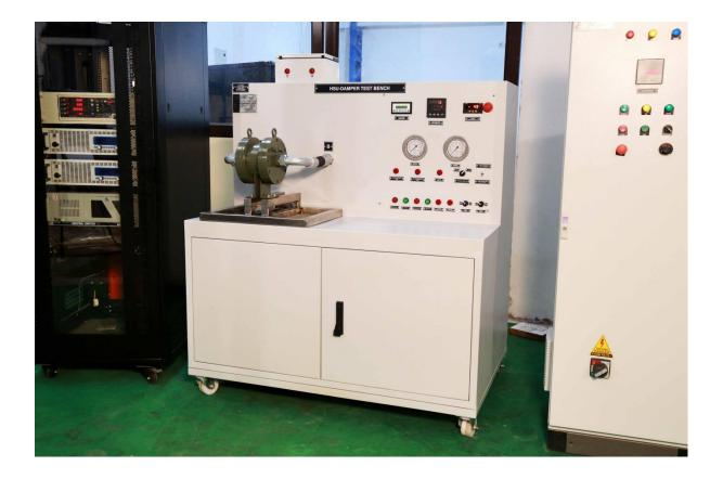
Damper test bench is a high performance test equipment to test the damper assembly of the main HSU unit. Testing to be perform to check the Differential pressure creating capacity of the damper assembly.
