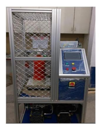
The Test Rig is Pneumatic System use to fill the Carbon dioxide in cylinder at a pressure of 3400psi and at temperature 160 F can be set. This machine is very well known for its robust working which will be very helpful in the Aviation Field.
