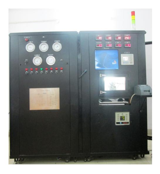
This unit is developed to check the Continuous Operation of CNG Regulator by conducting cycling test of 50,000 cycles as per ISO 15500-9:2001 (E). At different test pressure & temperature by pressurizing & depressurizing the component. Leak testing at high pressure is also done.
