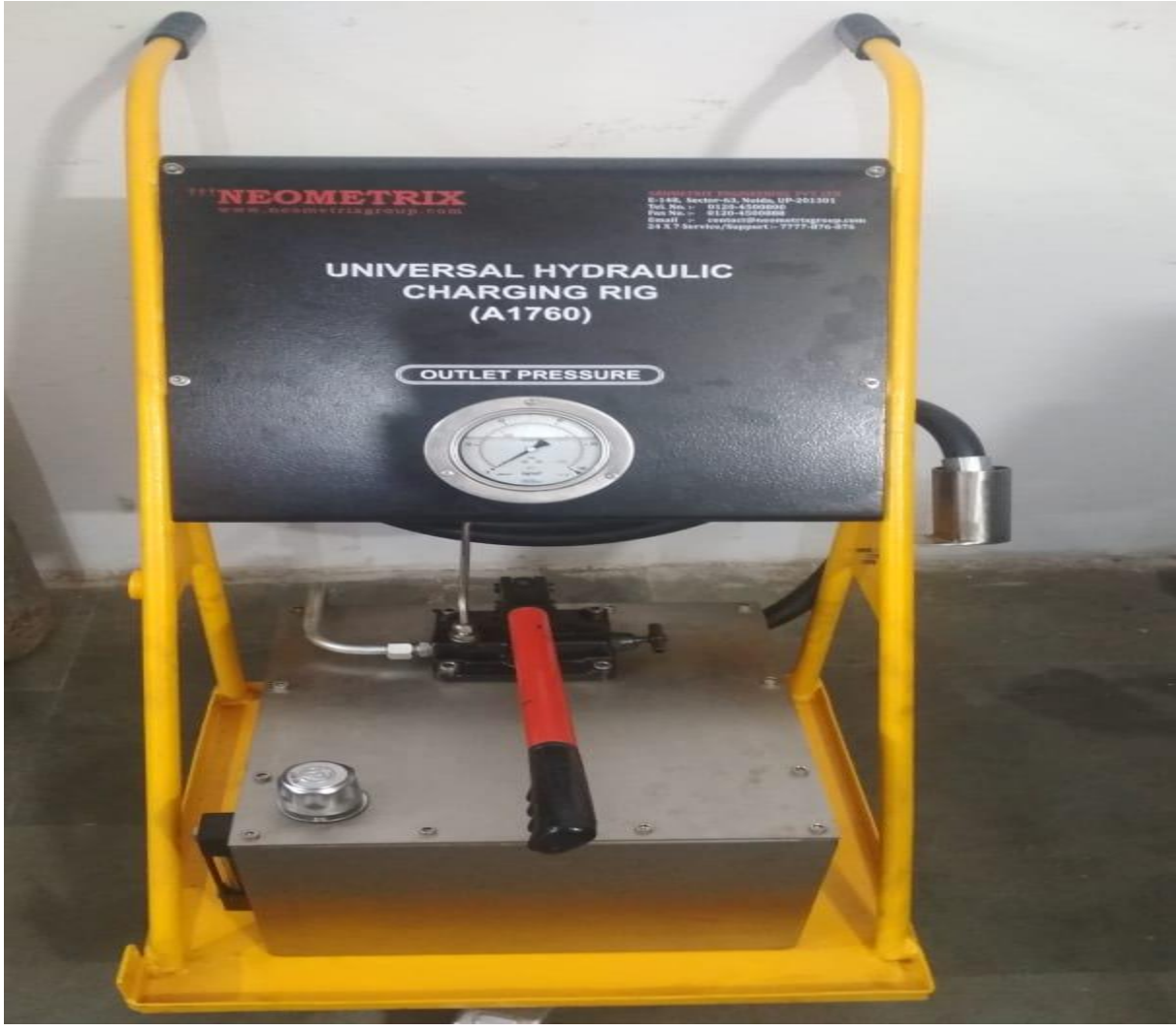
UNIVERSAL HYDRAULIC CHARGING RIG (A-1760)
