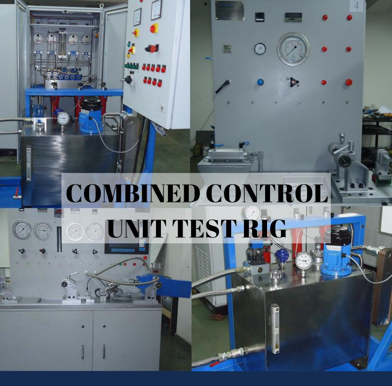
The Test rig is used for testing servo hydraulic actuator. It used for testing helicopter and fighter plane components. It is fully computerized system with the software which can control up to 120 testing sequence. There is also custom built report generation system. It can Test any servo hydraulic actuator used in aviation.
